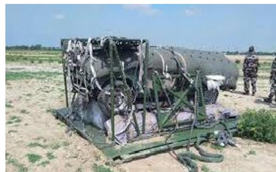
System consists of a platform and specialised parachute system. The parachute system is a multi-stage system which comprises of five Main canopies, five Brake chutes, two Auxiliary chutes, one Extractor parachute and platform is a metallic structure made up of Aluminium or steel alloys.
