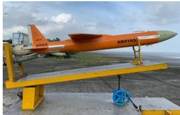
ABHYAS is capable of fully-autonomous flight and runs on a gas turbine engine.
